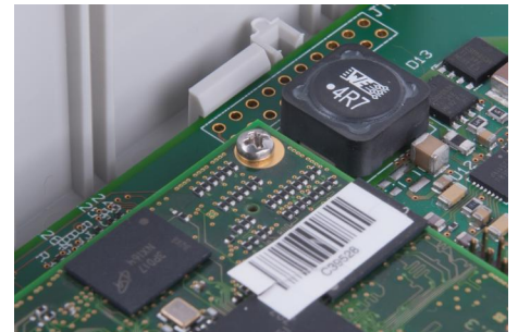
Depending on the design, optional screwless latching of the PCBs
