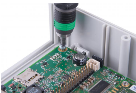
PCB mounting in the base and lid
