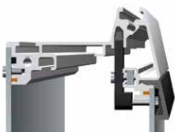
Front panel installation screwed from front
