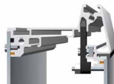
Front panel installation with stud bolts
