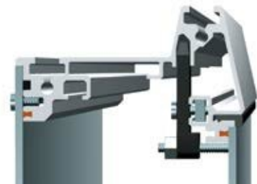
Front panel installation with stud bolts
