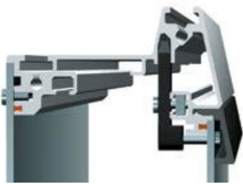
Front panel installation screwed from front
