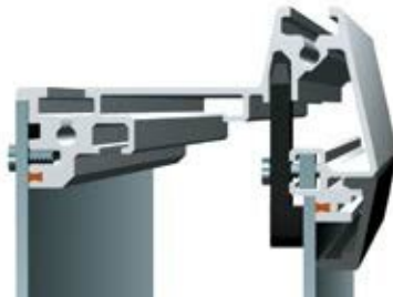
Front panel installation from rear
